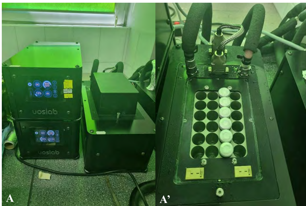
Supplementary Figure 1. Photochemical reaction set-up: UOSlab Miniphoto photoreactor (A and A').
